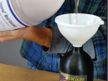
3. Fill Kwikee® sprayer no more than 2/3 full (24 oz/709 ml) maximum with a release or sealing agent that is clean and free of foreign particles.
