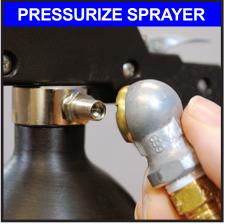
5. Charge sprayer with compressed air using a standard air chuck. Hold air chuck on valve stem until you hear the line pressure equalize with the sprayer.
